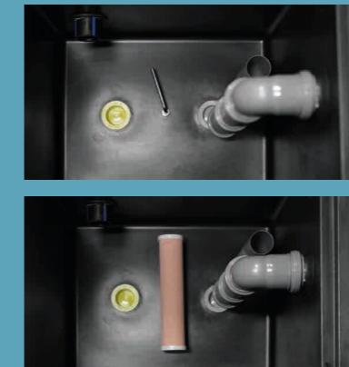
To do this, the screws at the bottom of the tank are removed and the ceramic filters supplied are screwed in hand-tight.
